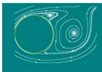
Fig. 14. The Streamlines in the Plane Z = 0.73d , Re = 260 , L = 7.5d .
