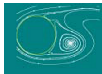
Fig. 15. The Streamlines in the Plane Z = 2.6d , Re = 260 , L = 7.5d .
